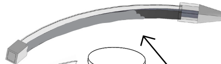
Even application of thermal adhesive glue using a brush
