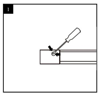
1. Using a flathead screwdriver(not included) pry off the plastic cap that covers the screw hole on the fixture than draw holes with a pen
