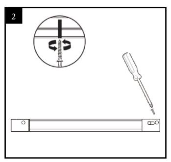
2. Place the fixture in the desired position and drive fixture mounting screws securely. Complete the mounting by putting back the plastic cap on the hole.
