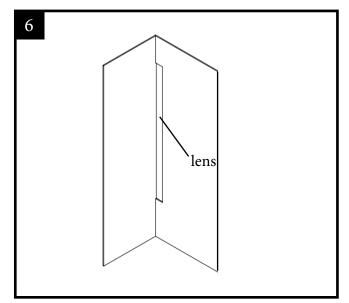
6. Once the enclosure is properly secured apply a fine quality plaster to give the final touch to the wall and then install the provided lens in place.
