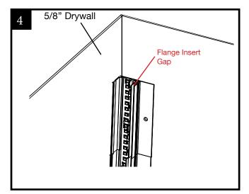
4. Locate the gap on the inner side of the end module and install 5/8" drywall with appropriate screws in aesthetic finish. Note: this should be along the side of the channel WITHOUT the flange insert gap.
