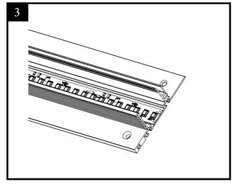
3. Install the tape light in the channel after testing it with the provided standard preciseLED driver and removing its back adhesive covering. Accommodate in the end module the extra tapelight that cannot be trimmed down to the desired length.
