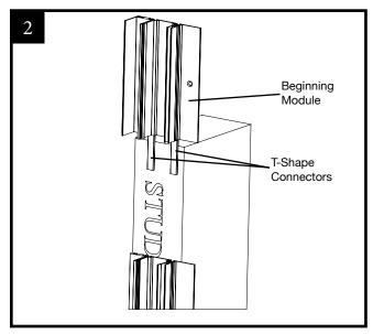
2. Attach Beginning and end modules(Provided) at each end of the channel by means of T-Shaped connectors(Provided).
