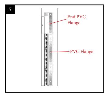
5. Install the provided PVC flanges into the gap along the remaining open side of the ZENLITE channel and end modules (indicated in red) for smooth edge finish after spackling and plaster. To mount the flange use M3 Flat head countersunk screws flushed with the 5/8" drywall/sheet rock.
