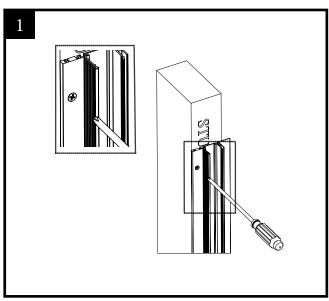
1. Place the ZENLITE® NC1 Perimeter channel on a corner stud aligning its holes with studs and trimming off the excess length at either side. Mount the channel with two M3x16 Flat head countersunk screws at each stud.
