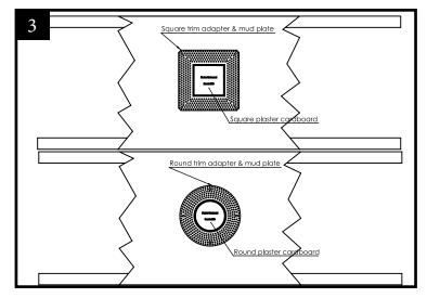
3. Mount the mud plate with trim adapter onto the drywall with provided 3/4" screws (ONLY for  $\geq 5/8$ " sheetrock). Insert the provided plaster carboard to prevent mudding inside aperture. Properly plaster onto the mud plate and drywall.
