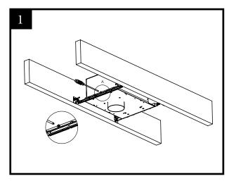
1. Install the housing to the ceiling joists or the drop ceiling T-bars with the adjustable bar hangers. Align the bottom of the end plate with the bottom of the ceiling support structure. Secure the fixture in desired position with locking-screw. (Note: bar hanger may be shortened to fit 12" framing or smaller by breaking at score lines.)
