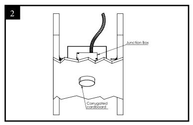
2a. Install the conduit into 1/2" trade size knock-out in the housing electrical box and connect all power line wires to the driver leads in accordance with NEC and local codes (see page 2 for detail wiring diagram).
