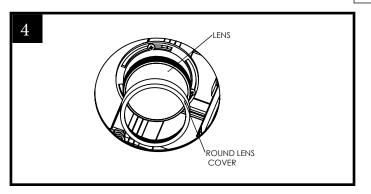
**4.** The default beam spread lens is  $60^\circ$ , and three additional lenses are available in  $45^\circ$   $38^\circ$ ,  $24^\circ$ ,  $15^\circ$ . Twist the lens cover to swap the lens. Use round lens cover for both round and square trim.
