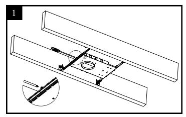
1. Install the housing to the ceiling joists or the drop ceiling T-bars with the adjustable bar hanger bars. Align the bottom of the end plate with the bottom of the ceiling supporting structure. Secure the fixture in desired position with locking-screw. (Note: bar hanger may be shortened to fit 12" framing or smaller by breaking at score lines.)
