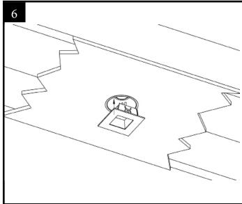
5. Mount the mud plate on the drywall using drywall screws. Properly plaster onto the mud plate and drywall.
