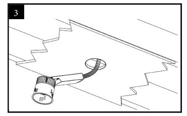
3. Install the conduit into 1/2" trade size knock-out in the housing electrical box and connect all power line wires to the driver leads in accordance with NEC and local codes (see page 2 for detail wiring diagram).
