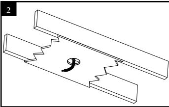
2.Pull conduit through housing opening and install drywall with 3 7/8" cutout.
