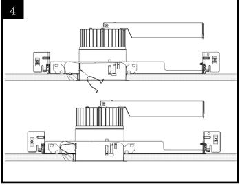
4. There are three groups of three slots on the fixture that account for varying heights of ceilings. Insert the three spring clips into the slots that allow the fixture to snap into the housing plate. Make sure the fixture is snug and has no room for movement.
