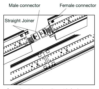
Remove the male connector, and connect the female connector to the male connector of next fixture. Join two fixtures together by the provided straight joiner and screws.
