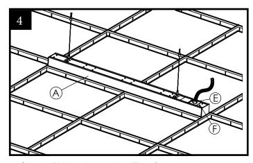
4. Secure BX knockout plate (F) to fixture
