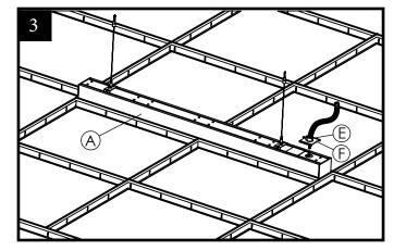
3. Install BX cable wire (E) into BX knockout plate (F), Wire BX cable wire (E) to fixture (A) using wire nuts.
