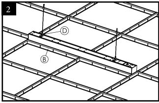
2. Secure the safety cable kit (D) to the fixture (A) and structure.
