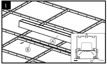
1. Ajust T-bar runner (B) to the fixture width. Raise fixture (A) above ceiling, place fixture T-bar support flange (C) onto flanges of T-bars runners (B) from the top.
