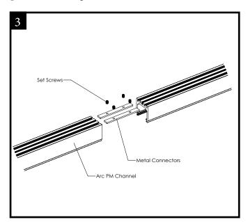
3. To connect two channels together, insert metal connectors into the slots at the back of the channel and hold them in place using set screws.
