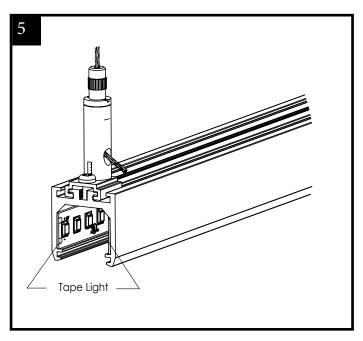
5. Drill a hole at the back of the channel wide enough to insert the feed wire. Feed the power to the tape withe the help of the pendant feed kits that are provided.
