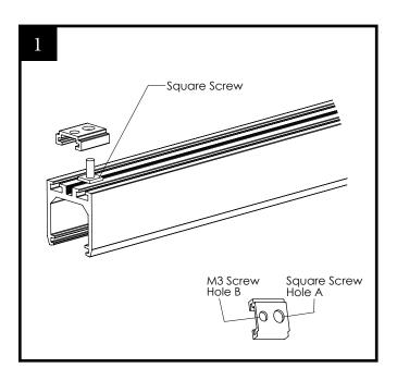
1. Insert the square screw into Hole A of the mounting bracket and slide the bracket to an ideal position\* through the slots on the channel
