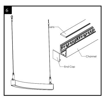
6. Install the provided arc lens and end caps in place. Insert the lens at the beginning of the channel and press it down along the edges
