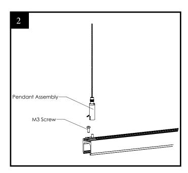
2. Use the M3 screw to secure the bracket in position and attach the remainder of the pendant accessories
