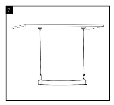
7. Mark the positions of the pendant kits on to the ceiling and drill holes to install the fixture to the ceiling. The finished installation is shown above.
