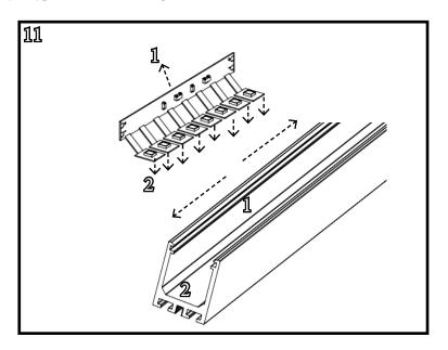
Step 1: Install the tape on the side of the channel.
