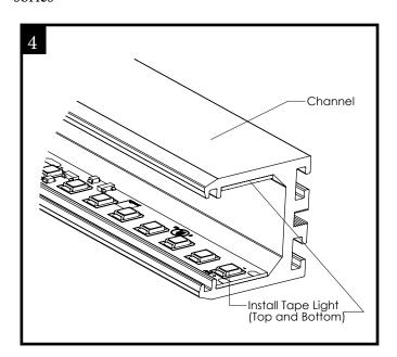
4. Install Tape light at the sides of the channel, using the standard PreciseLED driver, by removing the back adhesive.
