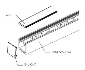
Note: Lead wire will either come out from side or back of channel
