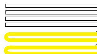
Note: The maximum length of a single channel is 8ft. For runs that are longer than 8ft, multiple 8ft channels need to be joined together by means of straight channel connectors. Seamless lenses can be shipped in rolls of lengths up to 40 feet.
