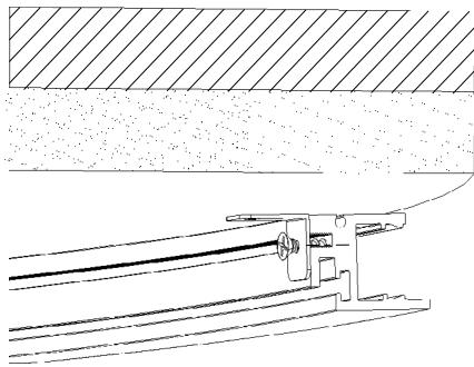
1. Attach Zenlite Mounting Clips to back of the Zenlite Float Arc channel with Zenlite M3 Screws, ensuring that clips are located to align with studs.
