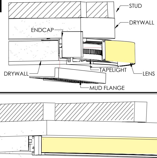
5. Install the Mud Flange into the appropriate Mud Flange Groove. Install Lens and Endcaps as shown. Apply plaster compound and spackle to complete installation.
