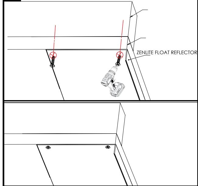
2. Use self-tapping Zenlite Screws to secure reflector to studs through dry wall.
