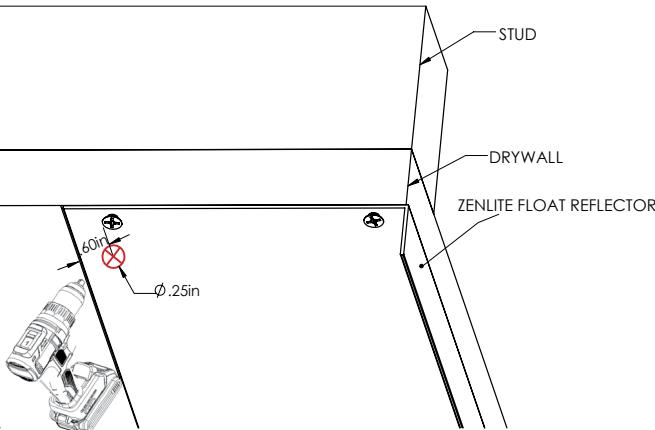
3. Once mounted drill a 1/4" hole in reflector approximately 0.60 inches away from the edge for the power feed to pass through.
