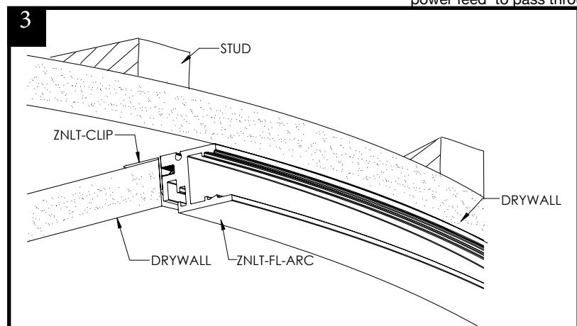
3. Install drywall over the Mounting Clips.
