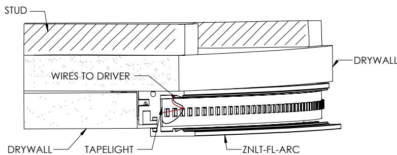
4. Remove adhesive backing on tapelight and center and place onto the back of the channel. (Wire the fixture to the driver according to the wiring diagram below.)
