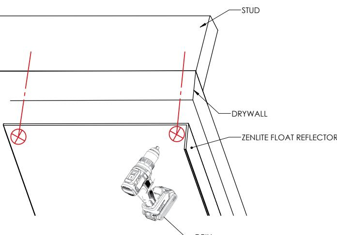
1. Drill holes in the edge of the Zenlite Float Reflector, aligning them with stud locations in the drywall ceiling.
